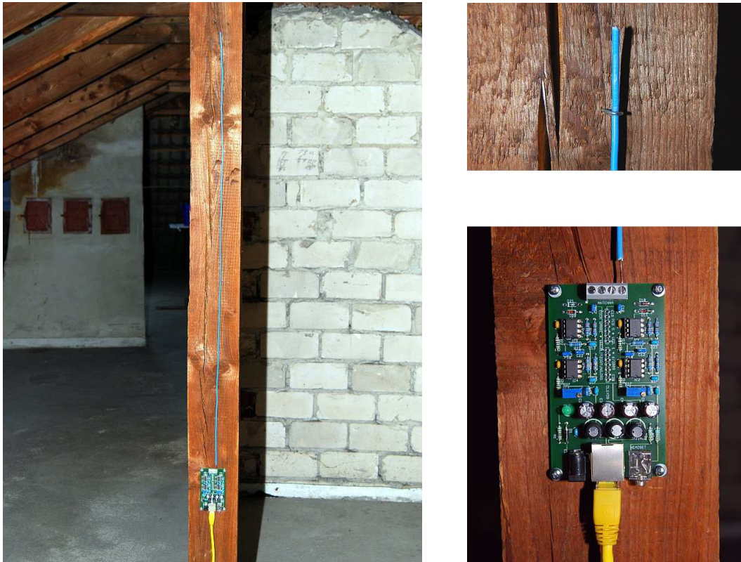
Figure 9: A wire of 1 meter length used as an electrical antenna.
