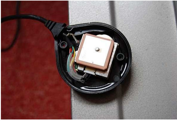
Figure 28: An EM-406A module embedded into the housing of a Fortuna U2, to the left, and embedded into a housing of a Navilock NL-303P, to the right.
