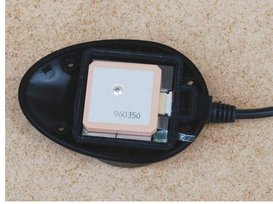
Figure 28: An EM-406A module embedded into the housing of a Fortuna U2, to the left, and embedded into a housing of a Navilock NL-303P, to the right.
